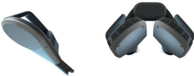
Figure 5: Single-coil (left) and double-coil (right) configurations, which served as the basis for the simulation models. Courtesy of BTL Industries, Ltd. Used with permission.
