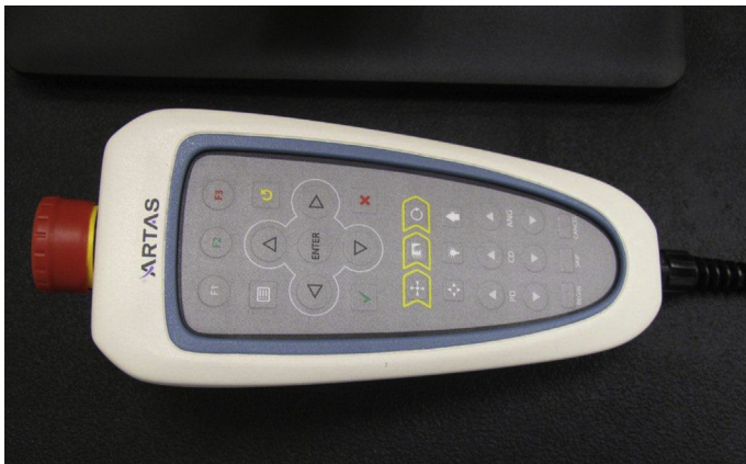
Fig. 5. The “pendant” that is held by the physician provides an ability to adjust the various harvesting parameters of the robotic device. There is an emergency stop button should the physician need to stop the machine while in motion.
