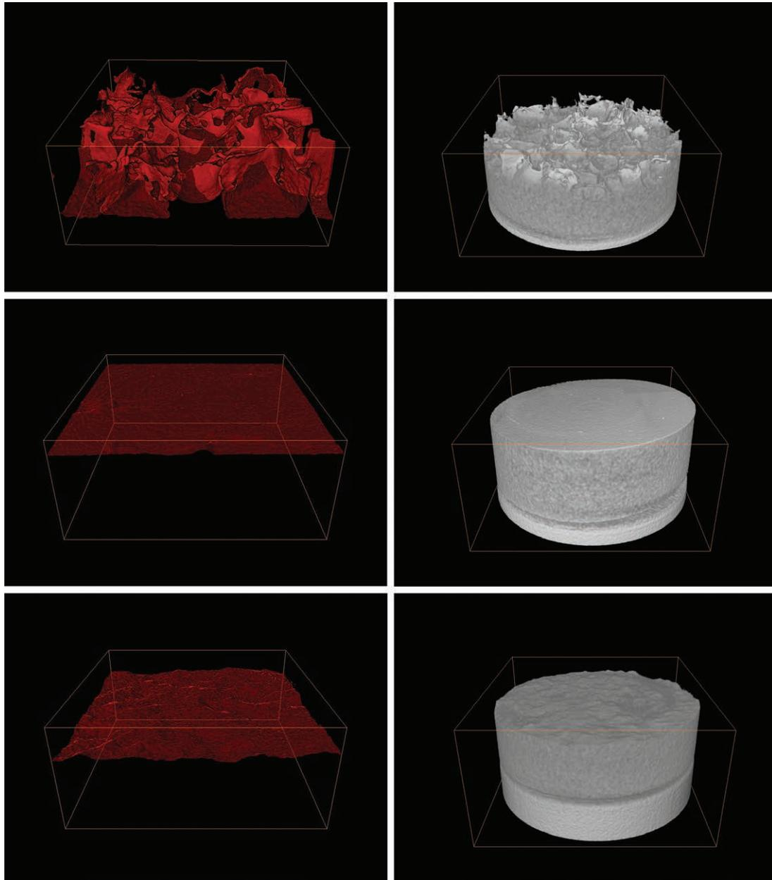
**Fig. 2.** Samples of three-dimensional cross-sections: extraction (*left*), and gray-scale reconstruction (*right*) from micro-computed tomographic analysis used for measurement of surface area/roughness. (*Above*) Allergan Biocell. (*Center*) Mentor Smooth. (*Below*) Motiva VelvetSurface.
