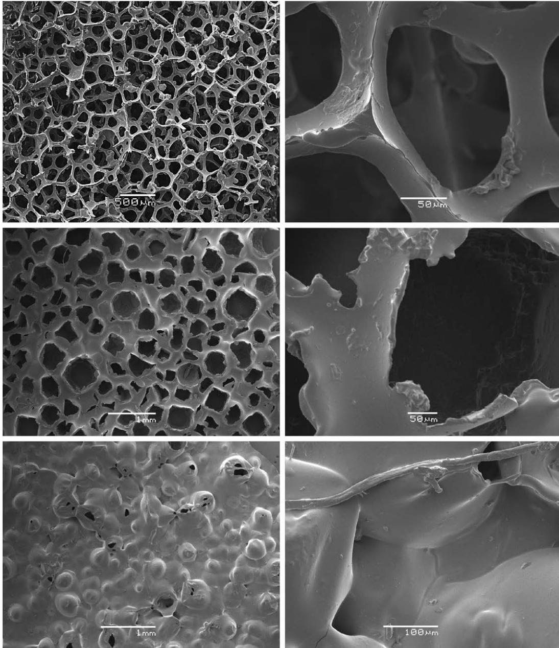
**Fig. 1.** Scanning electron micrographs of the surface morphology of implants studied at 25× and 400× magnification. (Above) Silimed polyurethane. (Center) Eurosilicone. (Below) Polytech POLYtxt.
