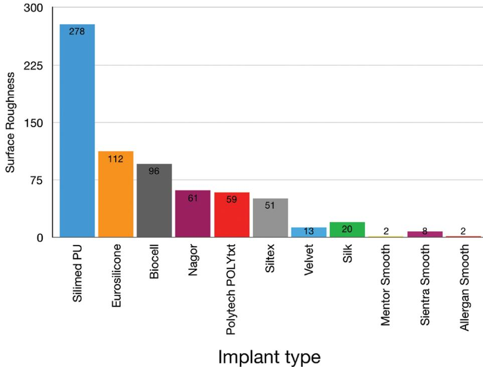
**Fig. 4.** Surface roughness for various implants studied. *PU*, polyurethane; error bars = SD.
