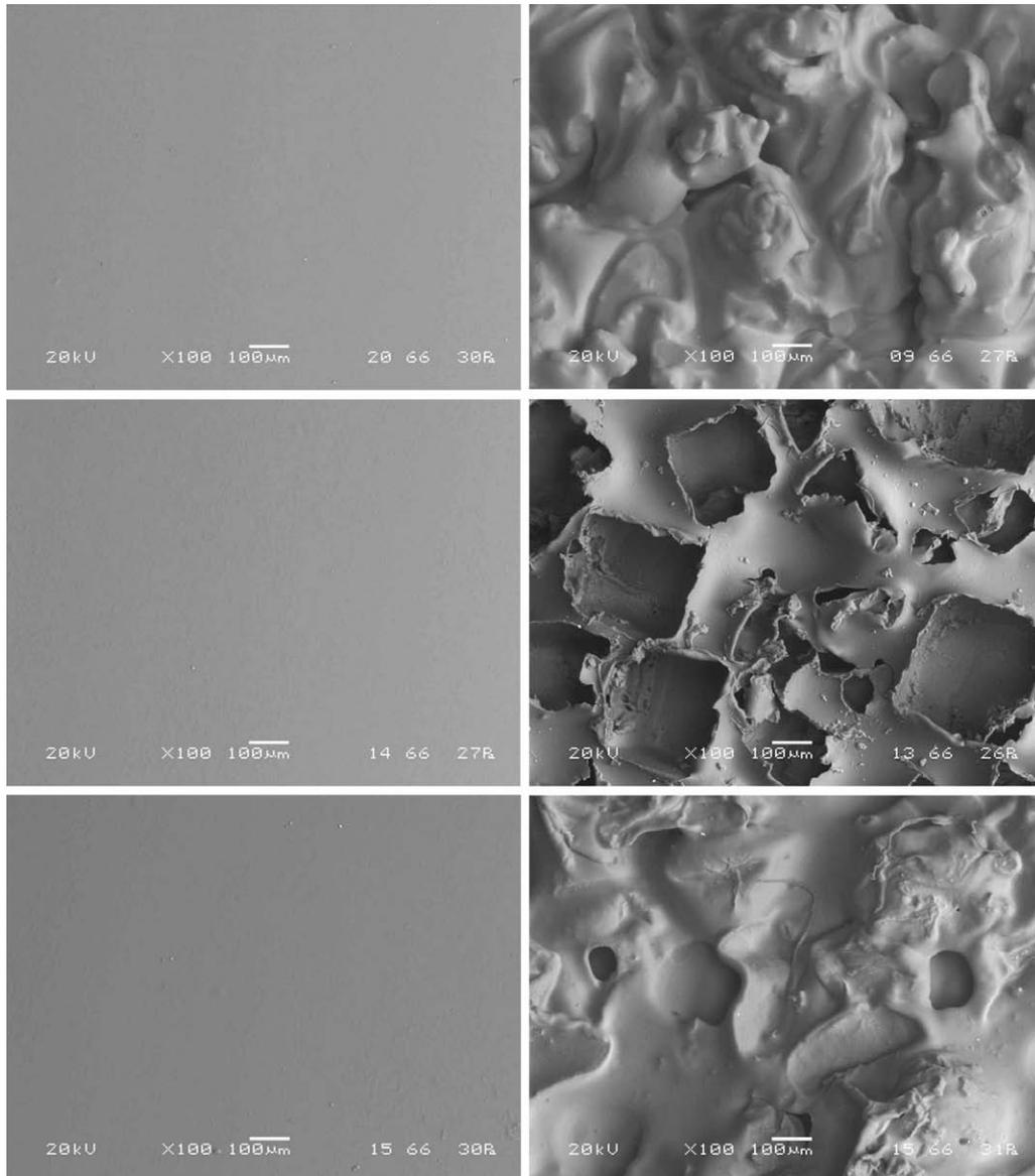
**Fig. 1.** Scanning electron microscopic images of smooth and textured implant surfaces. Mentor, Allergan, and Sientra smooth implant surfaces are represented by *left, above, center, and below*, respectively (original magnification, × 100). Mentor Siltex, Allergan Biocell, and Sientra TRUE Texture surfaces are represented in *right, above, center, and below*, respectively (original magnification, × 100). (Images provided by Mentor Corp.)
