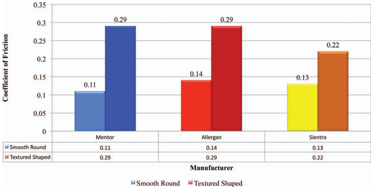
**Fig. 6.** Average coefficient of friction for Mentor, Allergan, and Sientra smooth and shaped breast implants. (Data from Rowe S. Ethicon AS&T Laboratories Protocol No. CP526. *Determination of Coefficient of Friction for Sientra, Allergan, and Mentor Anatomically Shaped, Gel-Filled Mammary Implants.* October 2013, Santa Barbara, Calif. October 31, 2013.)
